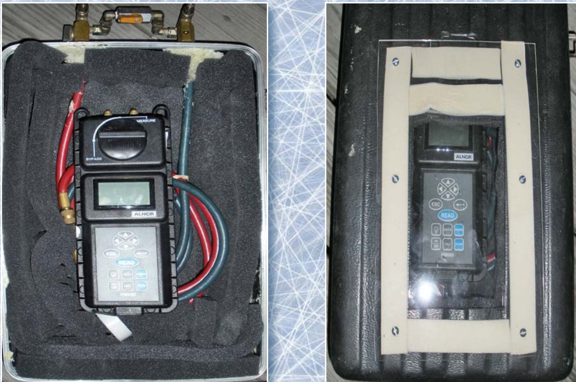
Figure 1. The testing apparatus described in the article, showing the completed assembly with the case open (left), and with the front closed to show the viewing window (right).
