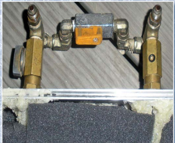
Figure 2. Detail views of the apparatus, showing the "primary loop" assembly inside the heated case ( left ), and the added bypass valve to purge the air from the secondary loop being plugged into the system ( right ).
