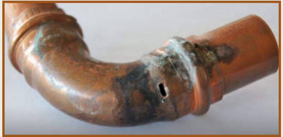
Pictured above is the section of pipe that was leaking inside the wall of a building.
