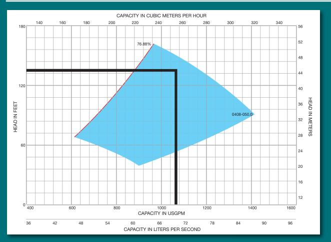
Meanwhile, the pump curve in the equipment submittal looks like this (also with the operating point added). While somewhat informative, the performance envelope curve is not much help in balancing the pump. It shows that the pump selected is capable of performing at design and it can operate down to about 70% of design load. It does not show RPM or impeller sizes.
