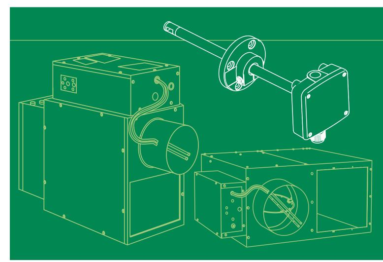
ach variable box or fan-powered box has a flow measurement tap which is connected from the measuring grid to the controller. The measuring grid has multiple measuring points and sends the average velocity pressure to the controller. The manufacturer marks high and low on the outside of the box. High is the total pressure and low is the static pressure. When connected to the controllers, the controller maintains the difference of high and low which is velocity pressure.
